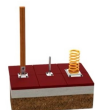
FIXATION SYSTEM Type X - Fixation system composed of a metal base bolted to the hard ground. The metal base is made of carbon steel sheet, with corrosion-resistant hot-dip galvanisation treatment of between 120 and 140µm thickness according to EN ISO 1461, which allows its placement without the plumb in direct contact with the ground. Its attachment to the plumb line is made by a quick clamping system increasing the longevity of the plumb line and its easy and fast replacement in case of need.
